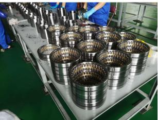
Multi-row cylindrical roller bearing, used for back-up rolls of rolling mills:
